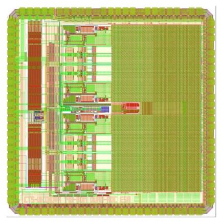
The microelectronics design group of our technical research center (CTS) at UNINOVA has been responsible for the design, layout, fabrication, and testing of a high-speed high-resolution QUAD-ADC Integrated Circuit (IC) under ESA contract no. 40001139457/22/NL/CRS.
